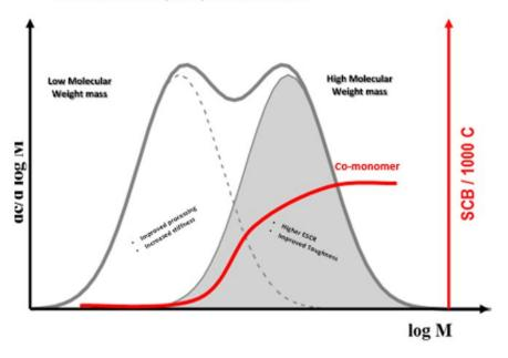
Safripol uses the Hostalen bi-modal process, now licenced by LyondellBasell to produce iMPACT100® PE100 pipe material
