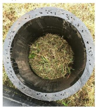
Bubbles caused by excessive moisture
